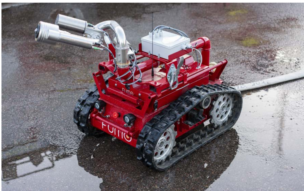
The Fumo fire-fighting robot with fire extinguisher and large-dimension hose.
